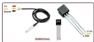
Gambar 2. Sensor suhu DS18B20
