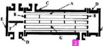
Gambar 2.6 Komponen Shell And Tube Heat Exchanger
