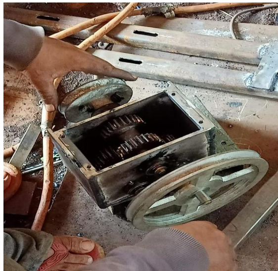
Percobaan kerja gear reverse
