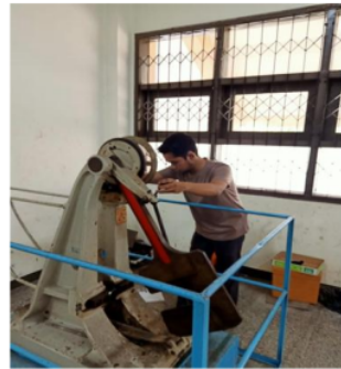
Gambar 2.8 Alat Uji Impact Charpy
