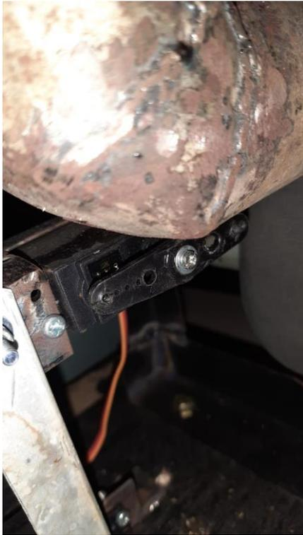
Gambar.6 Servo Pushing ball
