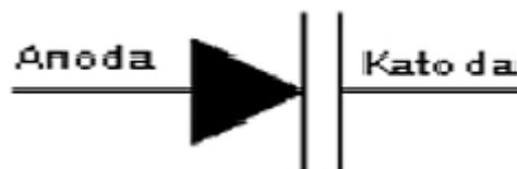
**Gambar 2.2.4(c)** Simbol Dioda Varactor
