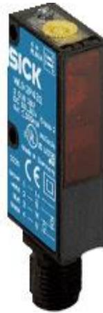
**Gambar 2.2.7(a)** Sensor Infrared Sick WL9-2N-131
