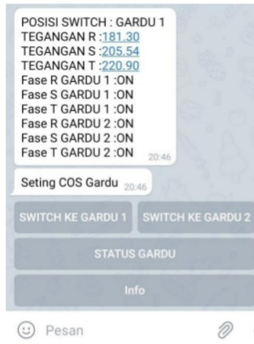
Gambar 11. Monitoring Tegangan Gardu 1
