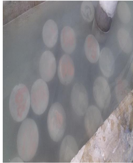
> Curing (Perawatan Beton)
