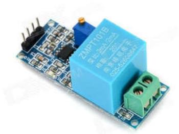
*Gambar 2.10.1 ZMPT101B Voltage Sensor Module*
