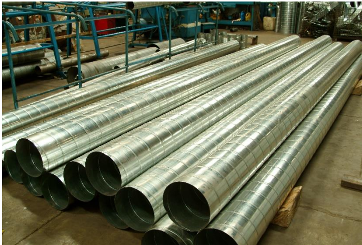
Lampiran 2 gambar spiral ducting
