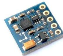
Gambar 2. Sensor Kompas GY-271 HMCL5883L
