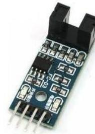
Gambar 3. Rotary Encoder
