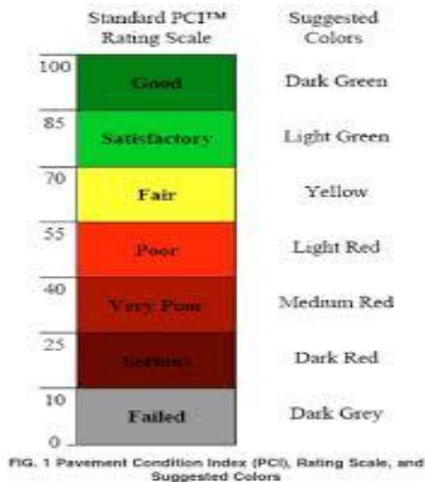
Gambar 2.22. Diagram Nilai PCI (Sumber : Shanin M.Y, Army Corp of Engineers USA1994)
