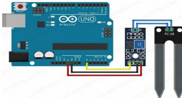
Gambar 3.9 Rancang Soil Moisture Sensor
