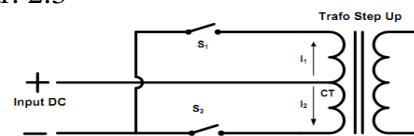
Gambar 2.2 Prinsip Kerja Inverter Push Pull
