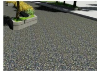
Gambar 11. Material Aspal Geopori
