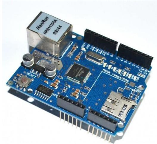
Gambar 2.7 Ethernet Shield
