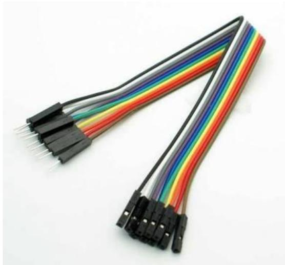
Gambar 2.13 Kabel *jumper male – female*
