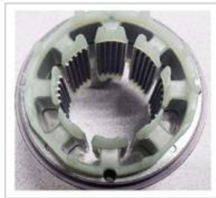
Gambar 2.11 Stator 8-Pole Tradisional
