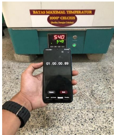
Temperatur solution heat treatment 540°C selama 1 jam
