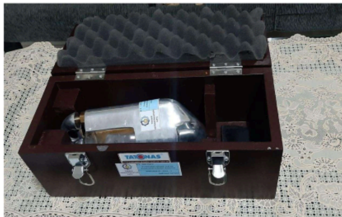
Gambar 3.9 Suspended Sampler USDH - 48
