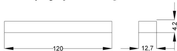
Gambar 19 Dimensi ASTM D790-07
