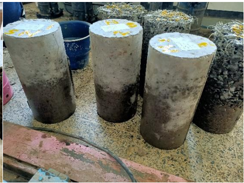
Benda Uji Beton Normal
