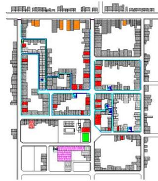
Gambar IX. Denah Drainase
