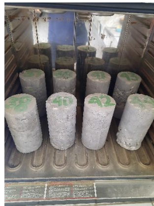
Proses Oven Uji Resapan Air
