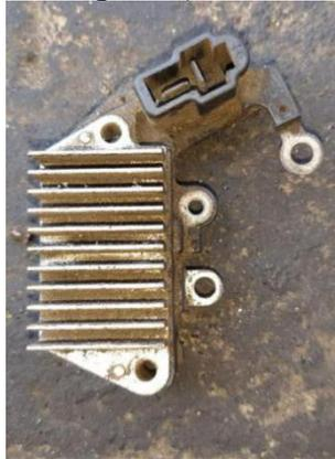
Gambar 2.5.4 AVR (Automatic Volt Regulator)
