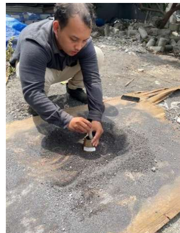
cornered to sand SSD condition
