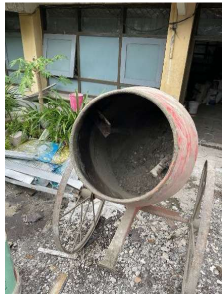
Stirring without water first so that the cement, gravel and sand are evenly mixed.
