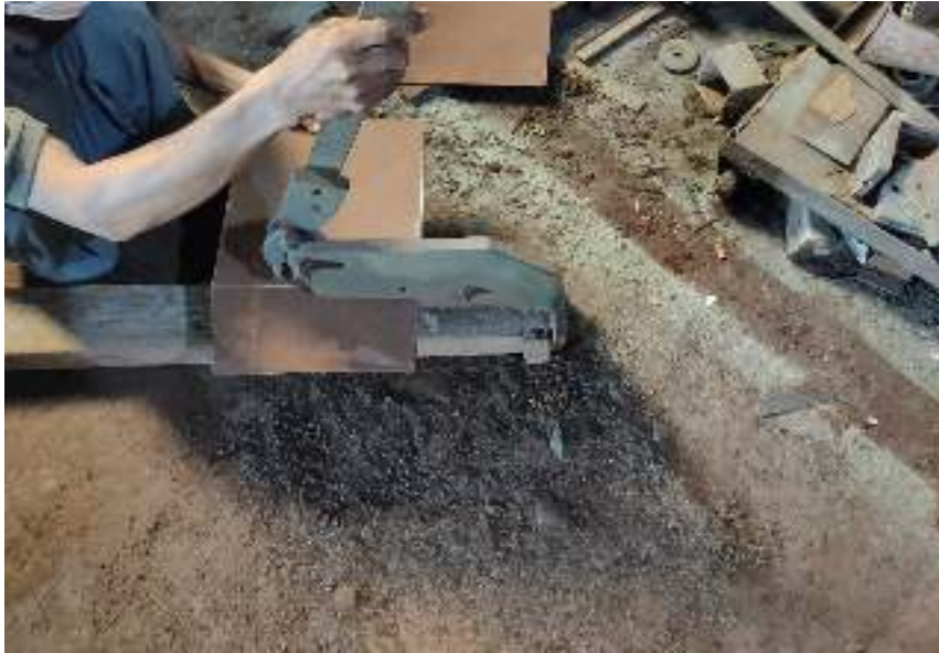
Proses pemotongan plat casing belt conveyor
