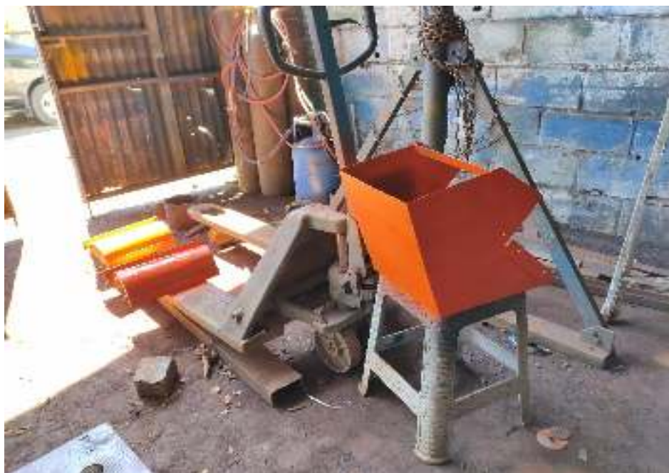
Proses pengecatan casing belt conveyor.
