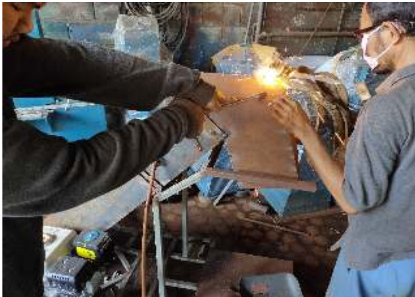
Perakitan casing belt conveyor.
