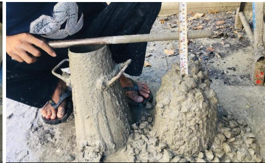
The measurement of slump value
