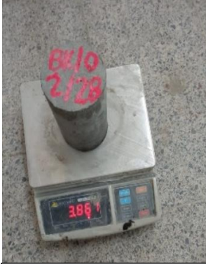
Weighing SSD concrete
