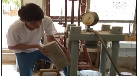
Putting the specimen to the compressive strength machine
