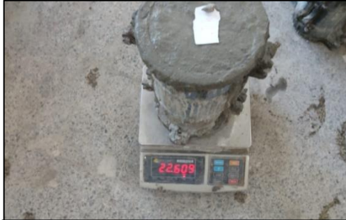
Unit weight test of fresh concrete
