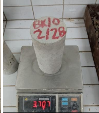
Weighing the specimen that has been backed
