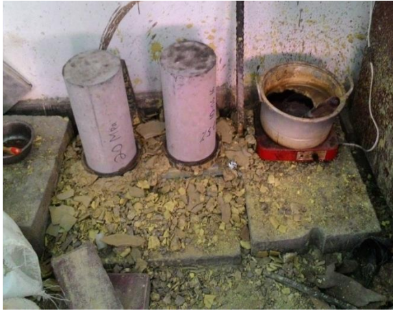
Gambar 5.16 Proses Caping Belerang
