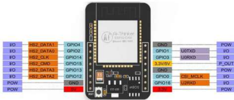
Gambar 2.7 ESP32 Camera Schematic Diagram
