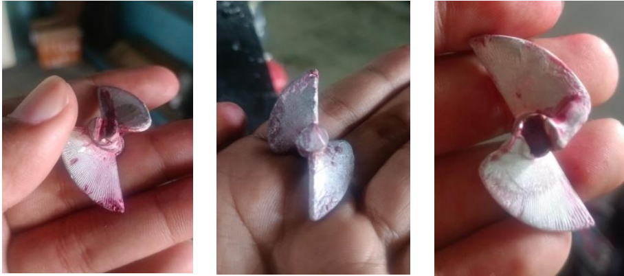
Proses Dye Penetrant Test
