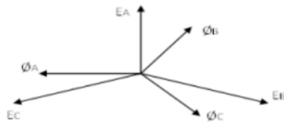
Gambar 1. Diagram Vektor Transformator Tiga Fasa
