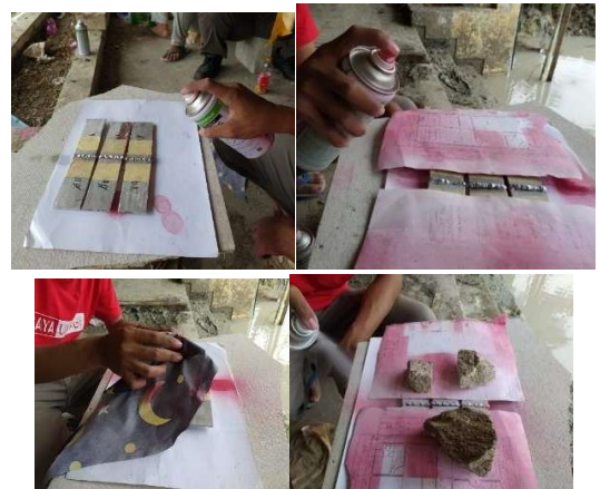
Gambar 4 Proses uji penetrant
