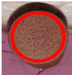
Gambar 6. Korosi Seragam (carboxylic 10 Hari)
