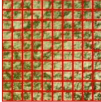
Gambar 10. Contoh Perhitungan Persentase Fasa Metode Point Count
