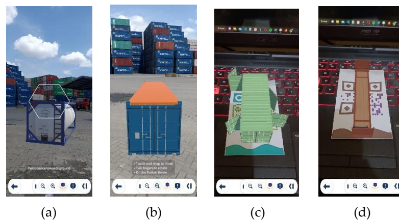
Gambar 8. (a) Markerless Tracking Isotank ; (b) Markerless Tracking Kontainer Open Top ; (c) Marker-based Tracking Kontainer Open Side ; (d) Markerbased Tracking Flatrack
