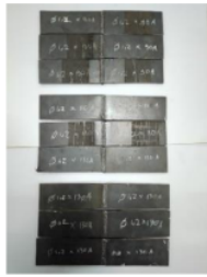
Gambar 4. Hasil Pengelasan Diameter Wire 1,2 Arus 90 A, 110 A, 130 A
