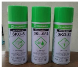
Gambar 5. Liquid Penetrant Testing
