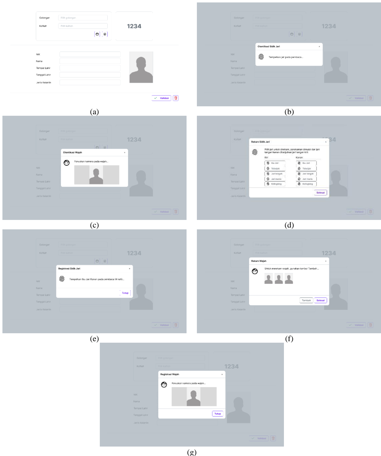
Figure 5 - Identity registration/recording interface; (a) main interface; (b) fingerprint recognition; (c) face recognition; (d) fingerprints enrollment; (e) enroll a fingerprint; (f) faces enrollment; (g) enroll a face
