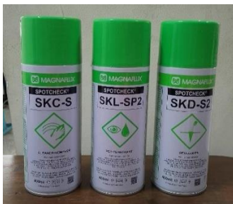
Gambar 5. Liquid Penetrant Testing
