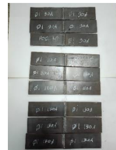
Gambar 3. Hasil Pengelasan Diameter Wire 1 Arus 90 A, 110 A, 130 A
