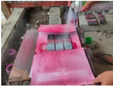
Gambar 11. Peyemprotan cairan Developer
