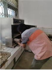
In the process of carrying out the compressive strength test of the mixed mortar test object, first prepare the cell phone to record the needle on the dial, then place the mortar and adjust the mortar to a parallel angle so that when the compressive strength test will get the maximum compressive strength. The following are the results of the compressive strength test on the mortar.
