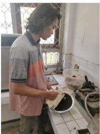
The process of testing mortar consistency by inserting 1/2 part and then cornered and after that put everything in and shaken again. Finally do the lifting simultaneously and measure the diameter. Here are the results of the consistency test.
