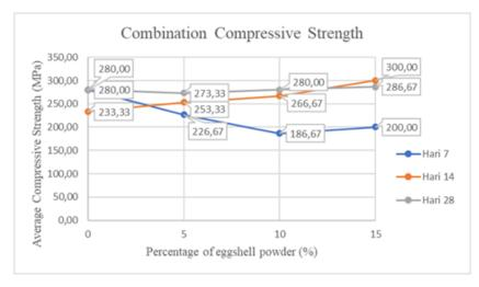
**Figure 6 Combination Compressive Strength**
