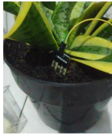
Gbr. 33 Pengujian Sensor Soil
