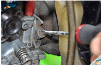
Gambar 5. Setelan gas karburator
