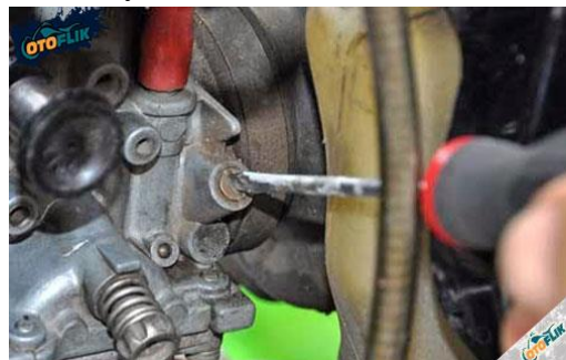
Gambar 5. Setelan gas karburator
