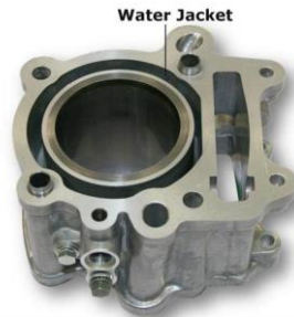
Gambar 7 Water Jacket Radiator
