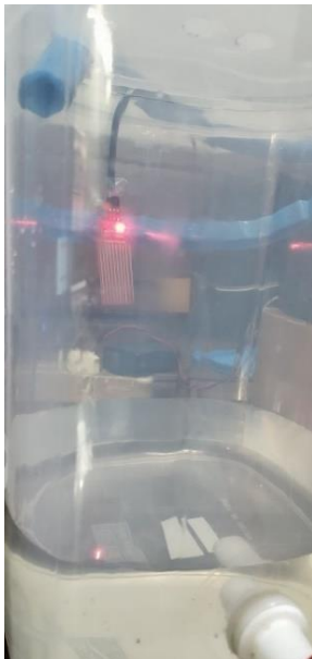
Gbr. 18 Sensor Water Level Belum Terkena Air
