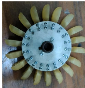
Gambar 5. Assembly runner dan sudu
