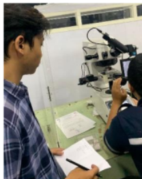
Gambar.6 Pengecekan micro vickres
