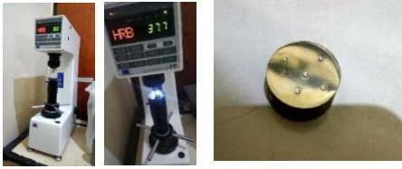
Gambar 4. Proses Uji Kekerasan HRB
