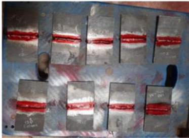
Gambar 6. Proses Pengujian NDT Liquid Penetran
