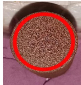
Gambar 21. Korosi Seragam (carboxylic 10 Hari)
